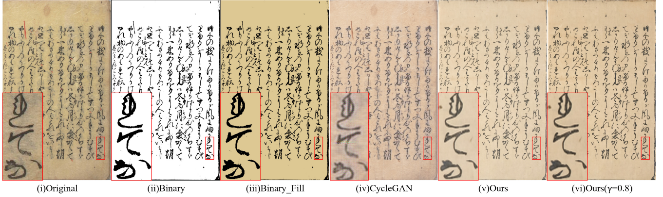
FIGURE 6: Restoration comparison for Tsurezuregusa . (i) Original image. (ii) Simple binarization using Otsu's method (non-learning baseline). (iii) Binary image with background correction, where white regions in (ii) are filled with the estimated paper color. (iv) CycleGAN-based restoration. (v) Proposed two-stage restoration guided by a binary mask. (vi) Proposed method with gamma correction ( \gamma=0.8 ) for enhanced visual contrast. Red rectangles highlight enlarged character regions for qualitative comparison.
